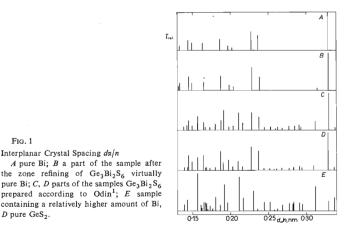
Fig. 1 Interplanar Crystal Spacing da/n A pure Bi; B a part of the sample after the zone refining of Ge3Bi2S6 virtually pure Bi; C, D parts of the samples Ge<sub>3</sub>Bi<sub>2</sub>S<sub>6</sub>
